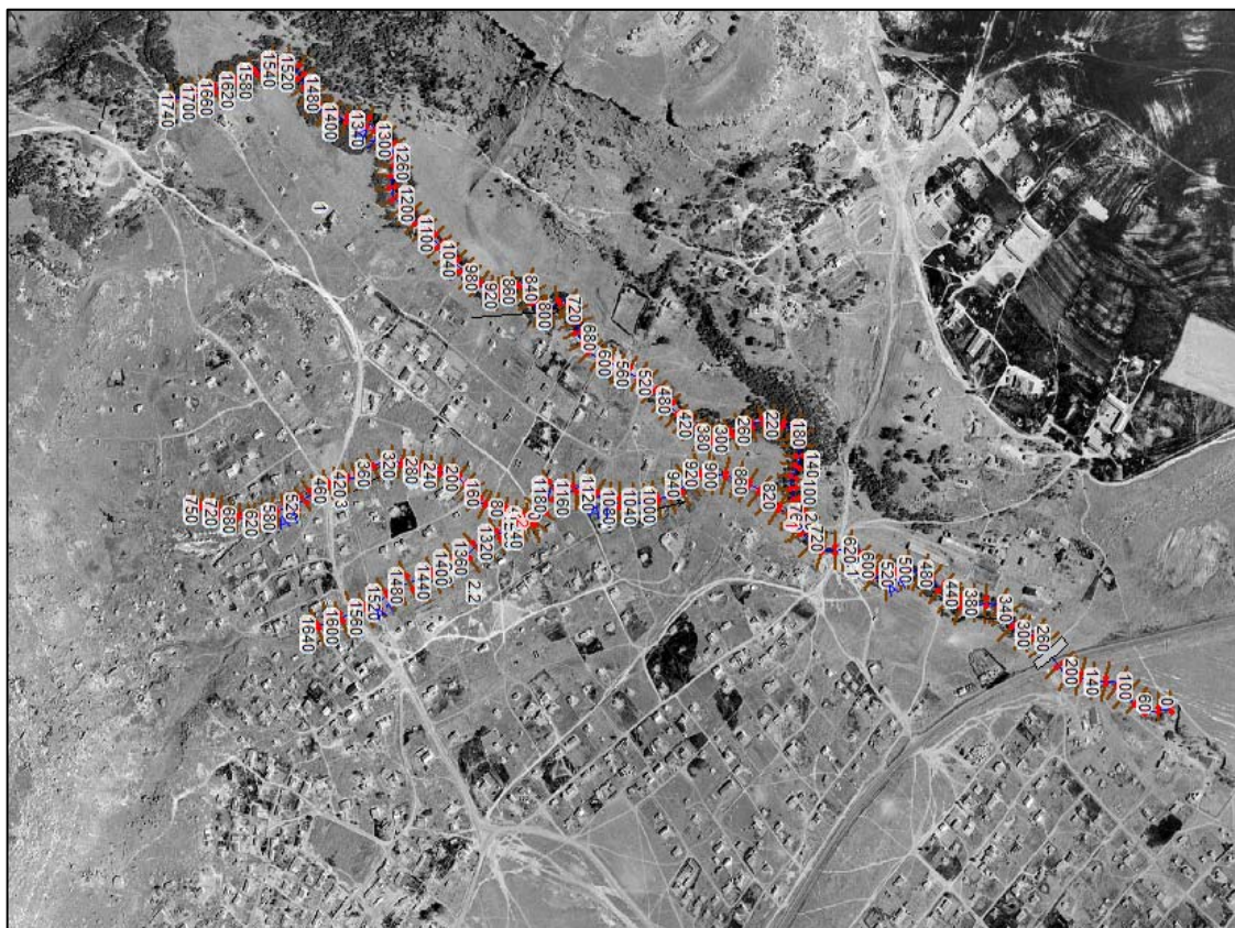
Figure 11.6: Numerical model set up for flood line determination
